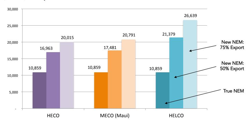
Note: System output calculation assumes (1) DC to AC de-rating factor of 0.81; (2) 475 sun zone (ie, 5.52 peak sun hours/day); and (3) 5% reduction for suboptimal tilt/ orientation. Current retail rate from HECO Companies Monthly Effective Rate Summaries at:
