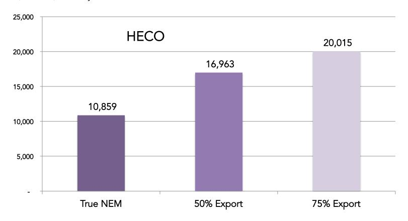
Note: System output calculation assumes (1) DC to AC de-rating factor of 0.81; (2) 475 sun zone (ie, 5.52 peak sun hours/day); and (3) 5% reduction for suboptimal tilt/orientation. Current retail rate from HECO Companies Monthly Effective Rate Summaries at:
