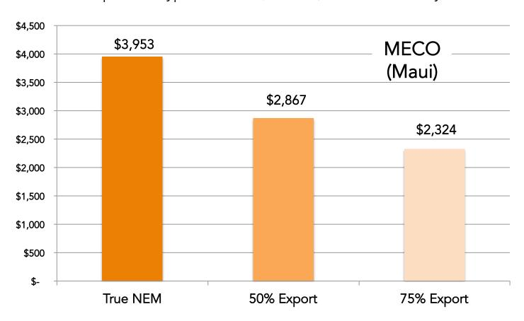
Note: System output calculation assumes (1) DC to AC de-rating factor of 0.81; (2) 475 sun zone (ie, 5.52 peak sun hours/day); and (3) 5% reduction for suboptimal tilt/ orientation. Current retail rate from HECO Companies Monthly Effective Rate Summaries at:
